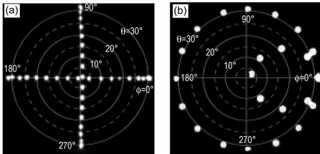
Fig. 3. Demonstration of Risley grating beam steering with a  $62^\circ$  FOR at 1550-nm wavelength. Note that individual pictures of the steered beam incident on an IR sensitive detecting screen were captured and superimposed.
