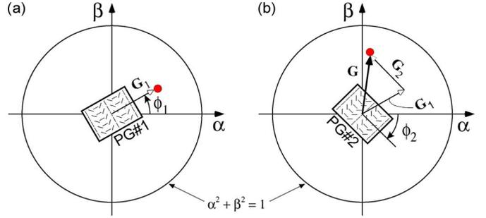
Fig. 2. Vector representations of PG diffraction in direction-cosine space: (a) the first PG diffraction  $\mathbf{G}_1$ ; (b) the second PG diffraction  $\mathbf{G}_2$ . The final direction can be expressed as a simple vector sum  $\mathbf{G} = \mathbf{G}_1 + \mathbf{G}_2$ .
