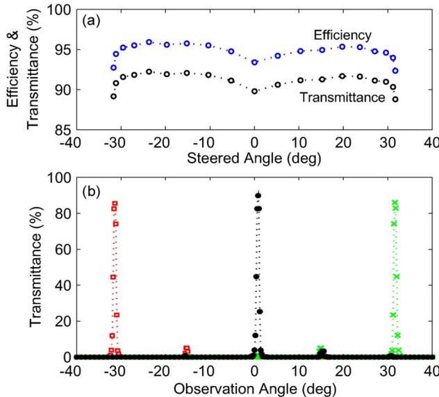
Fig. 4. High throughput from 92% to 89% of Risley gratings: (a) transmittance and efficiency of the steered beam across the FOR; (b) normalized power (transmittance) observed across the FOR  $\pm 40^\circ$  for three steering angles.
