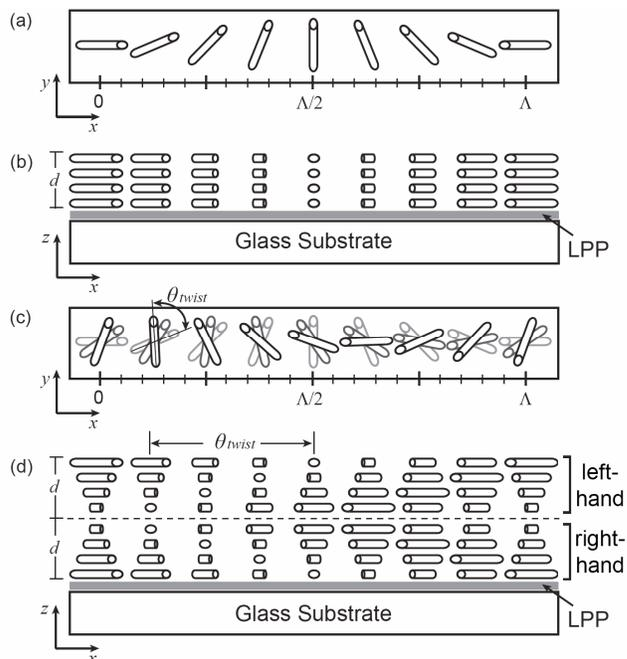
**Figure 1: Polarization Gratings (PG) – Basic geometry of a conventional PG, (a) top view & (b) side view; Achromatic PG with two chiral layers (opposite twist sense), (c) top view & (d) side view. The double-layered twist structure leads to efficient broadband diffraction by retardation compensation.**
