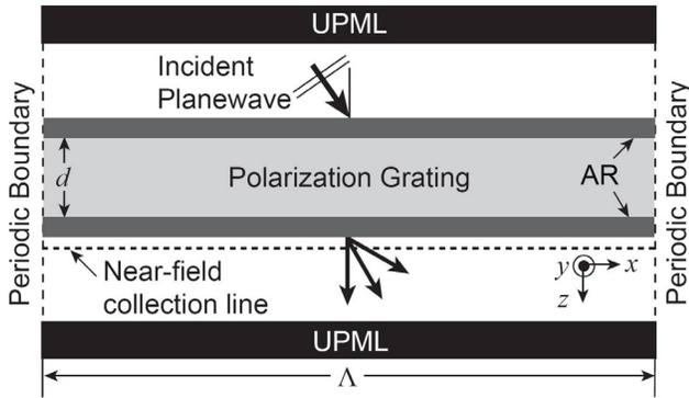
Figure 2: Layout of the 2D+ FDTD simulation space.
