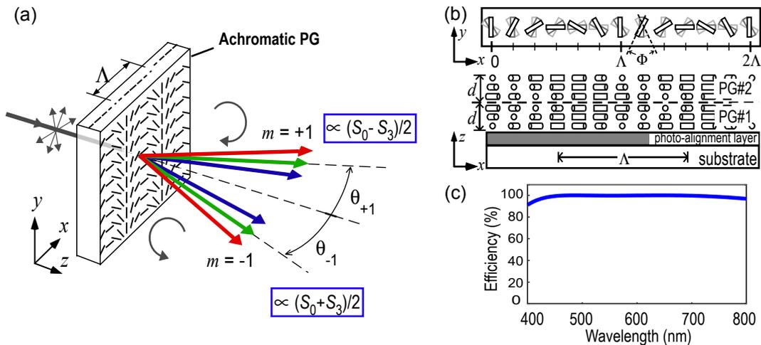
Figure 2. (a) Diffraction geometry and behavior of the Achromatic Polarization Grating (PG) (note only the  $m = 0, \pm 1$  orders are transmitted, according to Eqs. 2); (b) Nematic director profile of Achromatic PG and side-view (following Eqs. 1); (c) Total first-order diffraction efficiency ( $\Sigma \eta_{\pm 1}$ ).
