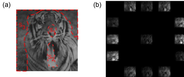
Figure 9. (a) One of the test image (high-resolution); simulated images are down-sampled as  $32 \times 32$  and manipulated to add polarization information. (b) Simulated dispersion spectrum; We can check the panchromatic image at the zero-order projection of dispersion spectrum
