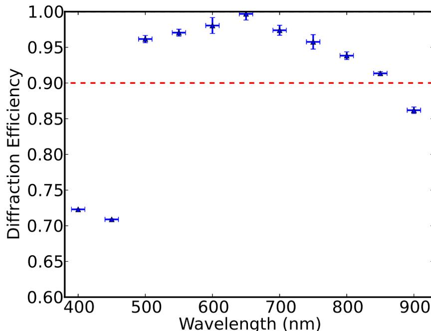
Figure 3. The diffraction efficiency of the visible PG. The red dashed line indicates 90% diffraction efficiency. The error bars in the wavelength direction represent the 10nm FWHM of the bandpass filters. A peak efficiency of 99.7% is achieved at 650nm.
