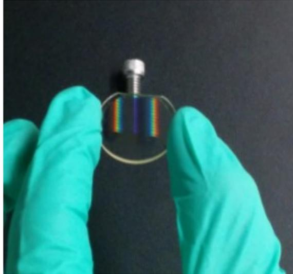
Figure 1. A photo of a visible PG, designed for testing at the University of Toronto. Where the PG is placed above the screw, images appear in the  $m = +1$  and  $m = -1$  orders. At bluer wavelengths the efficiency is not as high and the zeroth order can be seen at the center of the grating.
