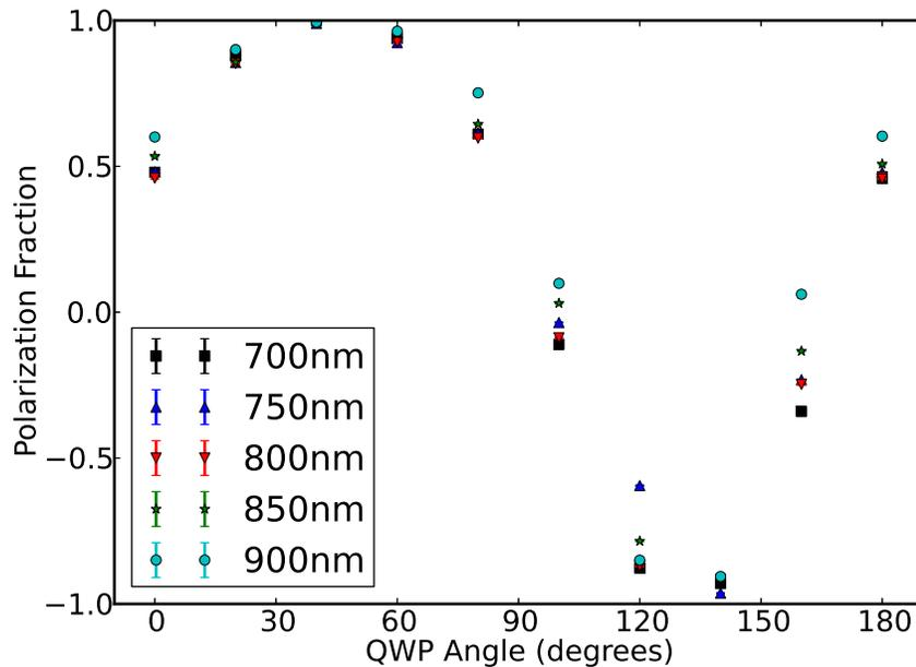
Figure 4. The modulation efficiency of the PG from 700 to 900 *nm*, measured every 20°. A peak modulation efficiency of 99.9% is reached at 700 *nm*.
