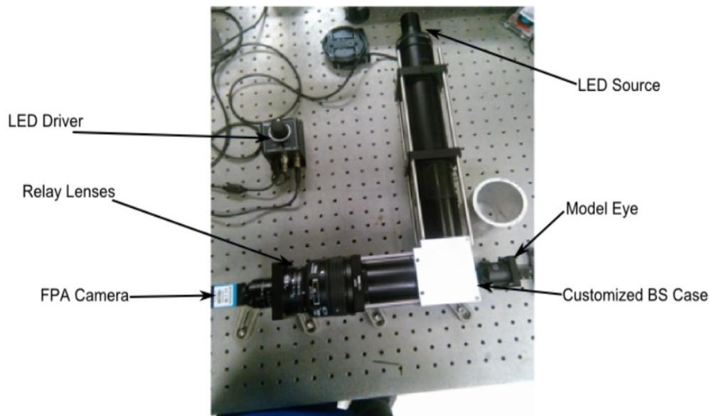
Figure 4. Experimental setup of SRIMMP system on an optical table
