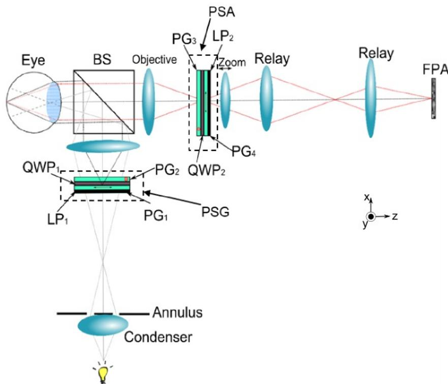
Figure 1. Schematic illustration of the snapshot retinal imaging Mueller matrix polarimeter setup.
