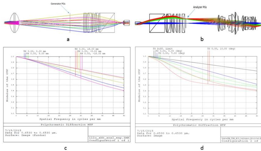
Figure 2. 2D sketches of a) illumination pathway and b) imaging pathway of the SRIMMP system, and the diffraction MTF curves of optics between c) PSG and retina, d) retina and FPA, with 4mm entrance pupil and 653 nm wavelength.
