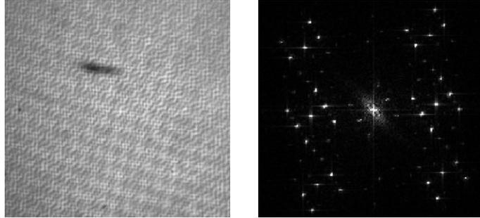
Figure 10. Polarization fringes acquired with a specular reflector as target and corresponding frequency domain pattern.
