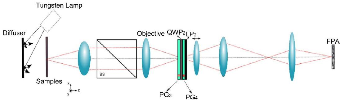
Figure 9. PSA calibration with calibration samples of known polarization states.
