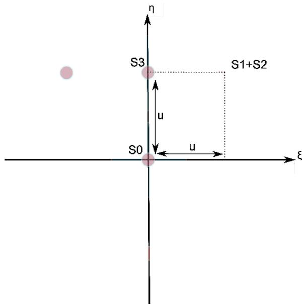
Figure 7. Ideal channel distribution of PSA in Fourier domain,  $\xi$  and  $\eta$  are Fourier domain coordinates for  $x$  and  $y$ .
