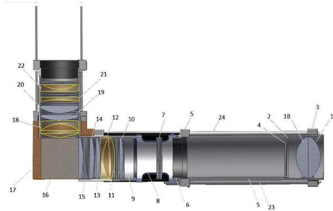
Figure 3. Cross-sectional view of the SRIMMP system assembly in Autodesk Inventor 2014.
