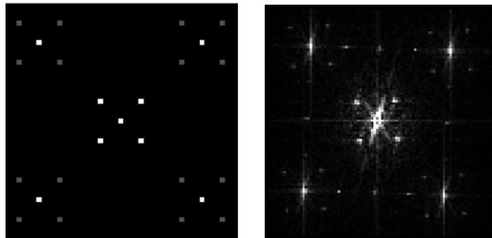
Figure 12. Frequency domain of the fringes in Figure 11, left: simulated; right: experimental.
