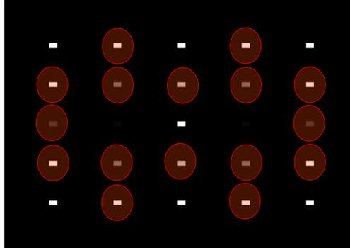
Figure 8. PSA frequency domain magnitude distribution, channels circled are created by defects.
